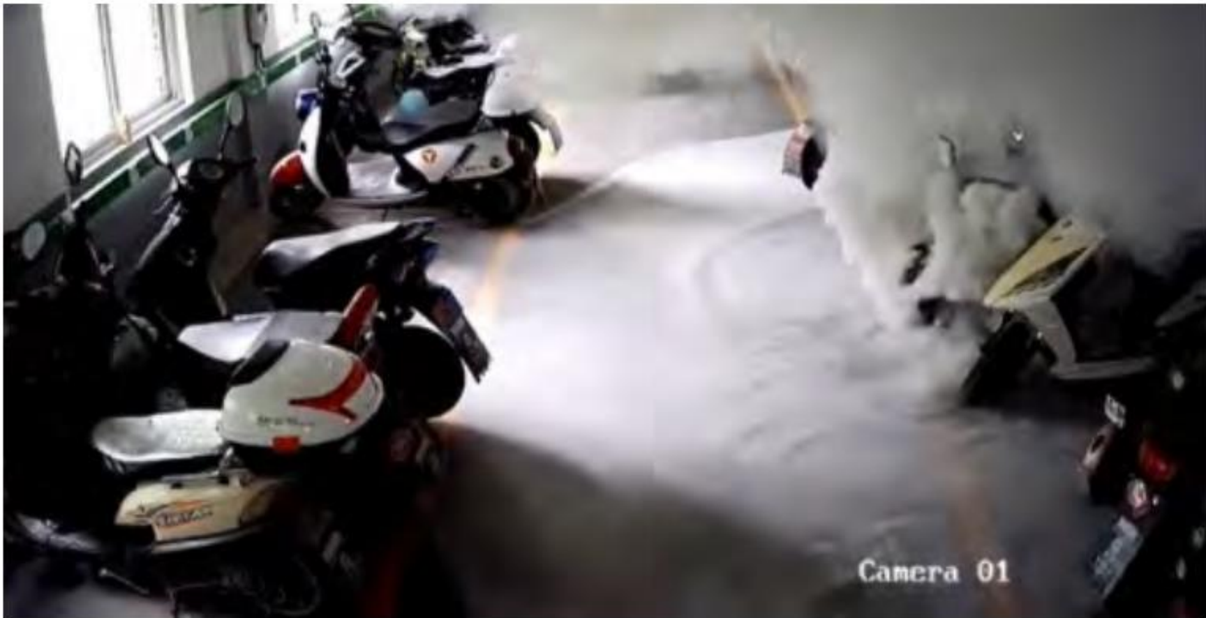
Figure 5 - Example of the different gases emitting from a battery during a thermal runaway event.
