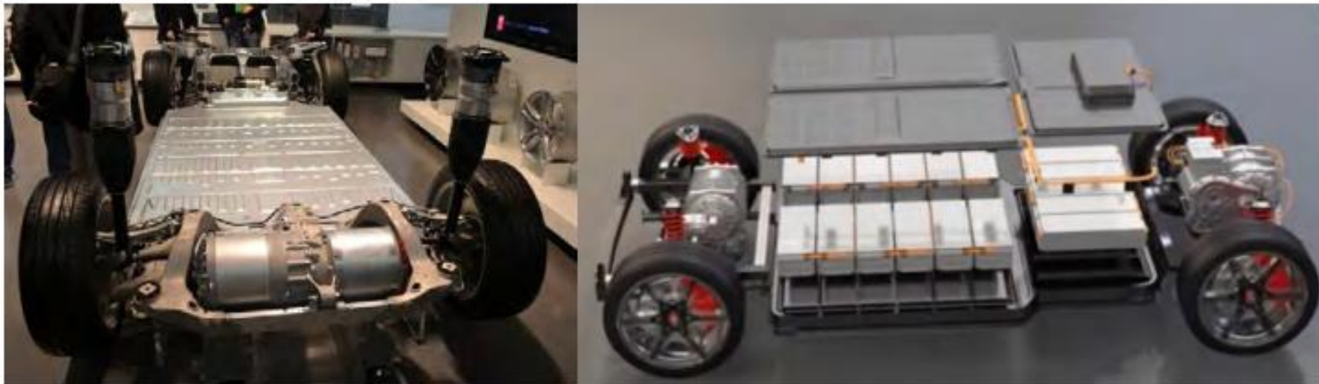
Figure 3 - Examples of the positioning of the battery packs in EVs, which is found in the chassis..
